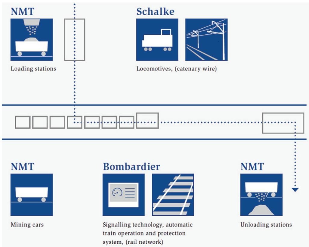
**Figure 6: Proven underground rail haulage system from Schalke, NMT and BT**
