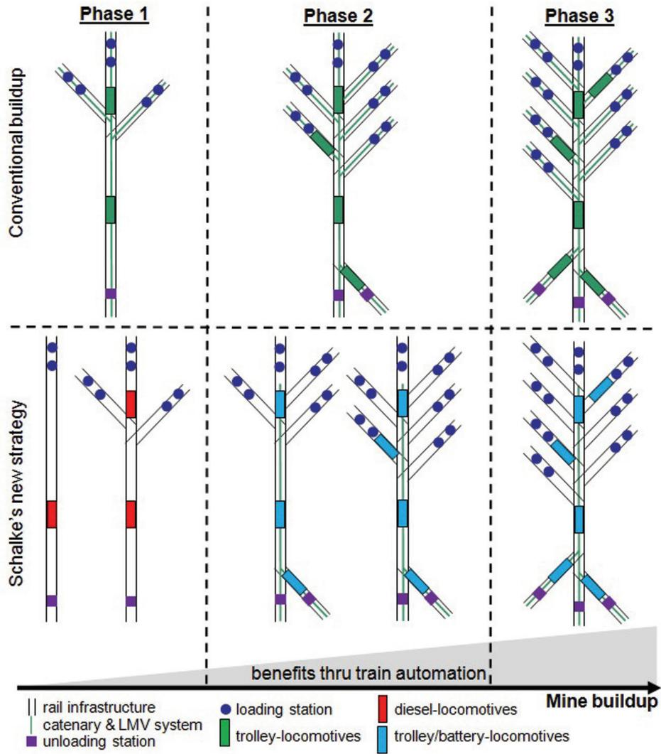
**Figure 4:** Conventional buildup of an underground rail haulage system versus new strategy based on Schalke's locomotive technologies
