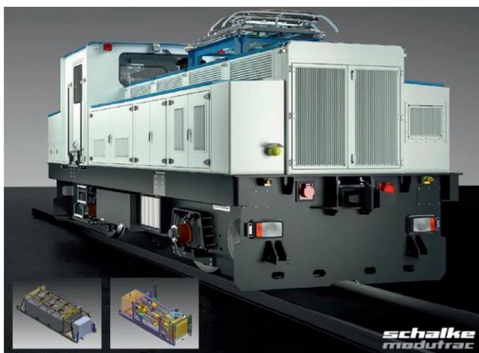
Fig. 8. MMT-M-270-BDE – Schalke's „ModuTrac“ mining locomotive running on battery or diesel power-pack with integrated trolley system
